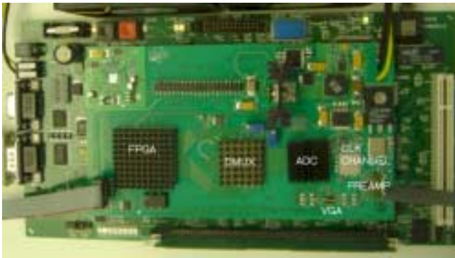
Fig. 5. Latest generation of SignalTrace™ hardware, which replaces most drive electronics functions. Note: Heat sinks obscure the FPGA and DMUX. most significant 8 bits of the ADC's 10 bits are used because 8-bit resolution is usually sufficient (HDD read channels typically have no more than 6-bits of resolution).
