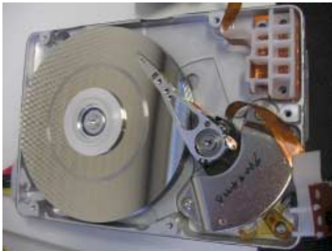
Fig. 1. The dull ring near the middle diameter of this spinning disk is the result of a head crash. The headstack shown is a new replacement from a donor drive. The flex circuit at the top of the picture is connected to the old damaged headstack. The new headstack's flex circuit (lower right) is connected to circuitry that replaces the drive's electronics, see section V.
